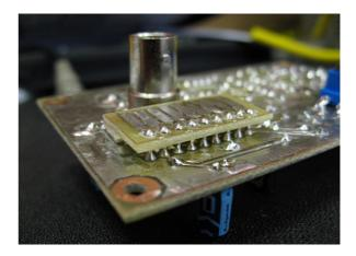
Regarding the Autoprobe pins we used a stack of PCBs to adjust the height of the pins, as shown on the picture... and it works !
