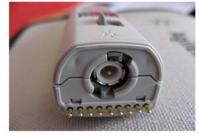
Just connect such a probe to a compatible scope and voilà, the probe is automatically recognized and powered. But from time to time you may want to use your probe with other test instruments, not equiped with an Autoprobe interface. For example we wanted to connect it to our spectrum analyzer and to a Lecroy waverunner scope. Is it possible? You bet yes...
