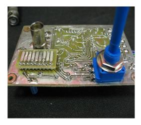
The RF connection is redirected from the probe connection BNC to a rear side BNC with a very short track (not 50 ohm but with minor impacts for the majority of applications as we are at the output of the active probe), allowing to connect it to your measurement instrument through a standard BNC/BNC cable. Don't forget that the equipment input should be 50 ohm.
