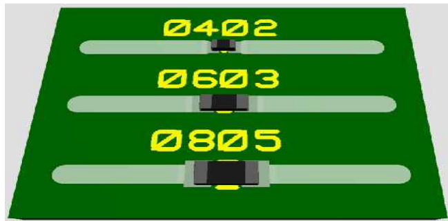
Impedance mismatches will be reduced if you select components with a package roughly the same size than the calculated track width. Here a 0603 package will be the better choice for this 0.9mm wide microstrip track.
