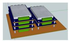
The SmartBrich modules are driven by a host system (microcontroller, DSP or PC, either embedded or remote) through the patented ultra-flexible SmartBus interface, compatible with SPI, USB, UART or I2C links. Open source software libraries provides an easy interface with any user-developed application in virtually any language: Labview, C, C++, Python, C#, Visual Basic, MATLAB/Scilab, etc.
